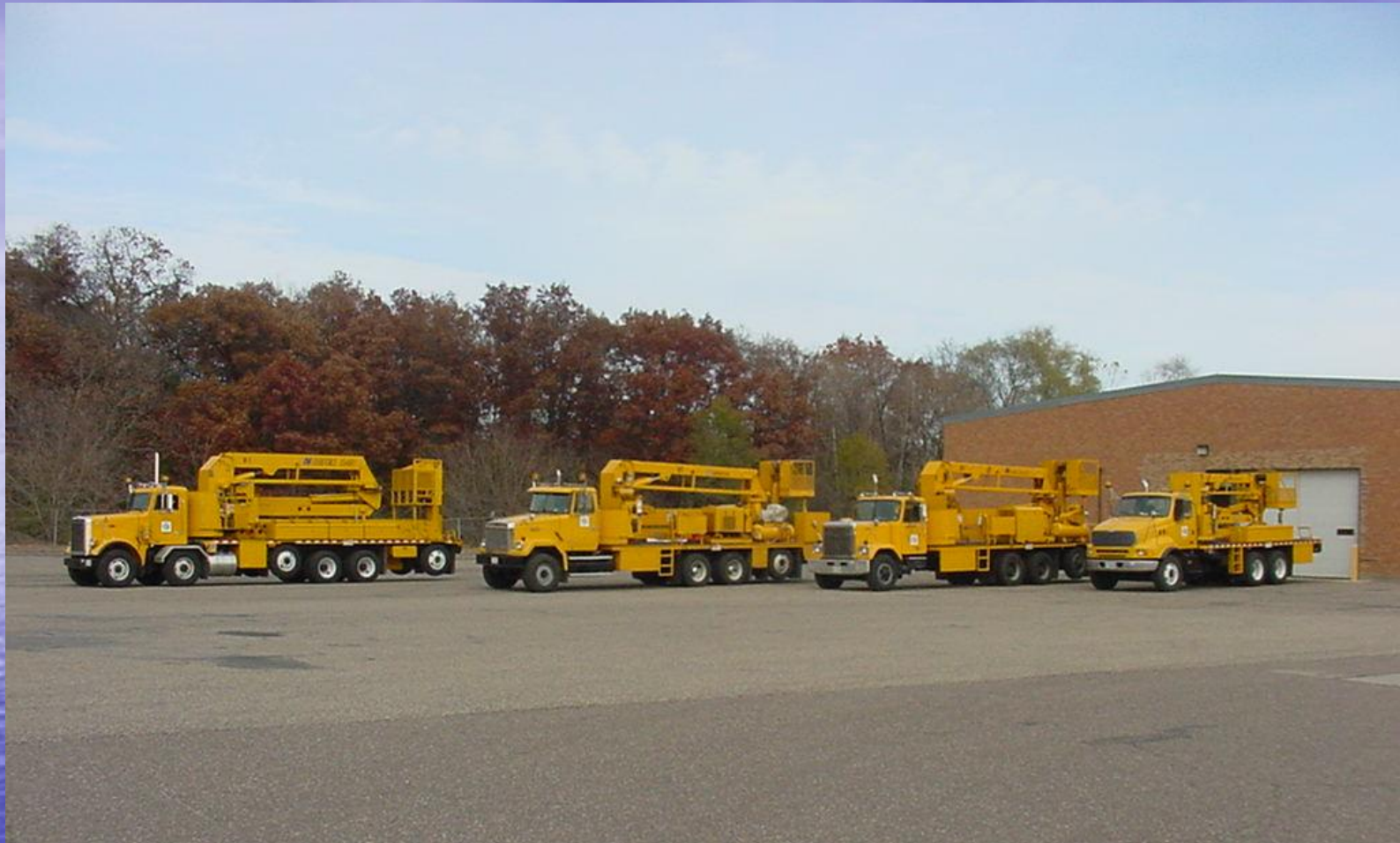
Under Bridge Inspection Vehicles (Snoopers)
